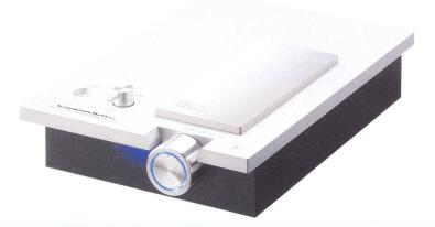
Luxman's stereo vacuum tube control amplifier, with a precision made brass, four gang volume control, featuring an in-built mute function. By touching the centre of the volume control, the sound mutes at once. Signal switching is performed by a golden switch immersed in a nitrogen container, located near the input terminals in order to maintain a low S/N Ratio.
